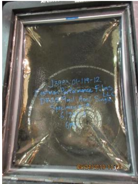
Photo No. 2 Post-test Specimen #1, Interior
