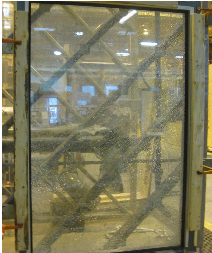
Photo No. 6 Test Specimen #53 Impacted with Center Punch
