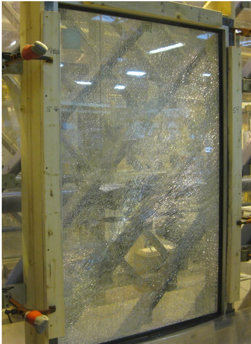
Photo No. 7 Test Specimen #54 Impacted with Center Punch
